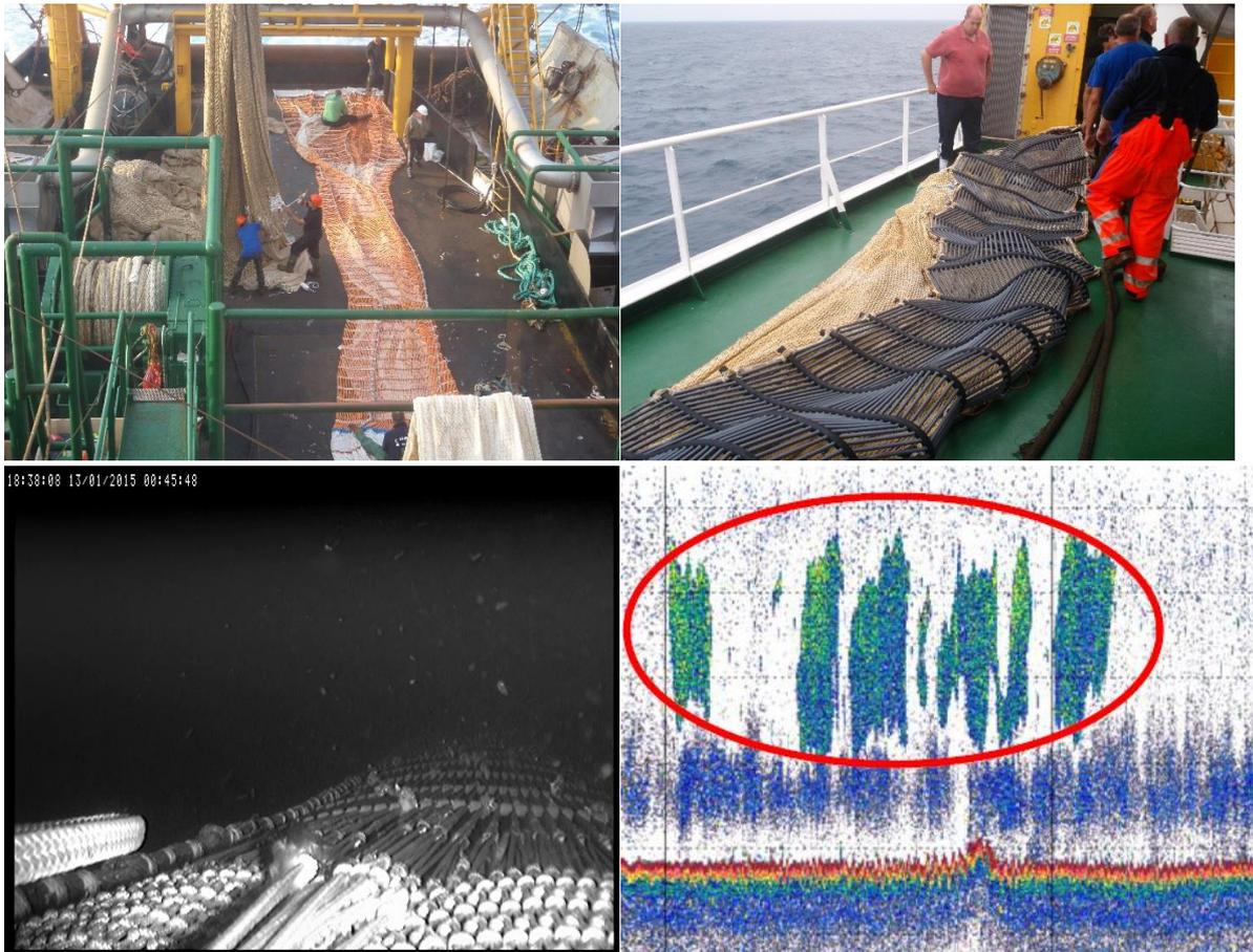
Left to right and top to bottom: Escape grids based on dyneema, escape grids based on dyeema with PVC cover, still from net camera showing a haul of boarfish and no boarfish escaping from the grid on SCH81 Carolien, acoustic identification of boarfish schools on SCH6 Alida.
