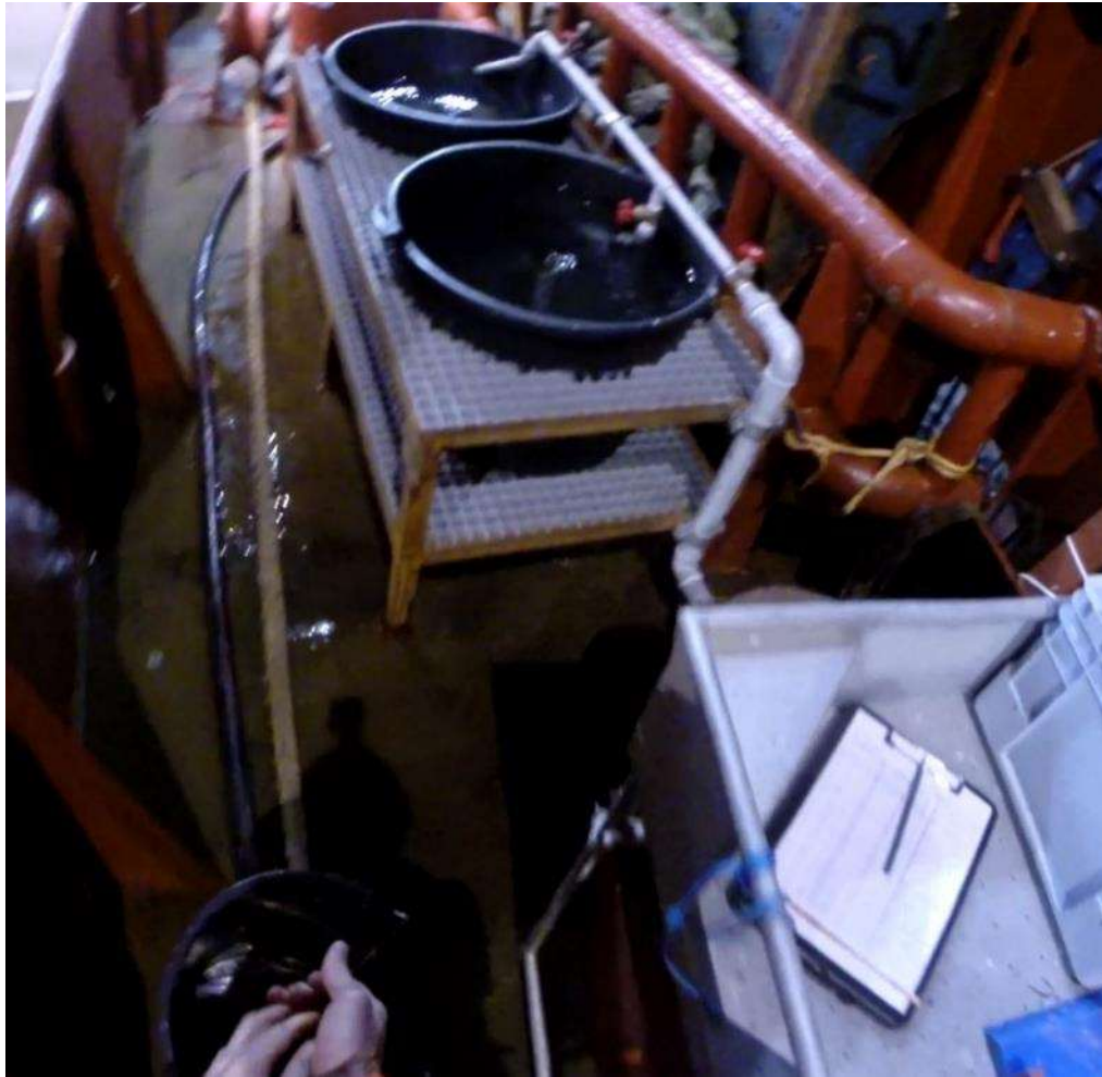
Figure 2.7. Fish condition monitoring tubs developed specifically for the research project. Each of the tubs contain flowing sea-water where fish can be held until vitality assessments can be carried out.
