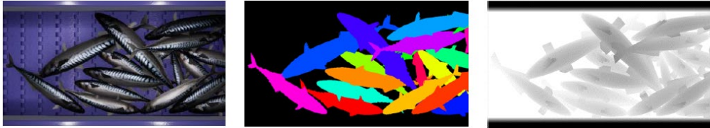
Figure 4.5.2.4. Generation of 3D model of mackerel on a conveyor belt (left), segmenting the fish into individuals (middle) and adding a field of depth (right).
