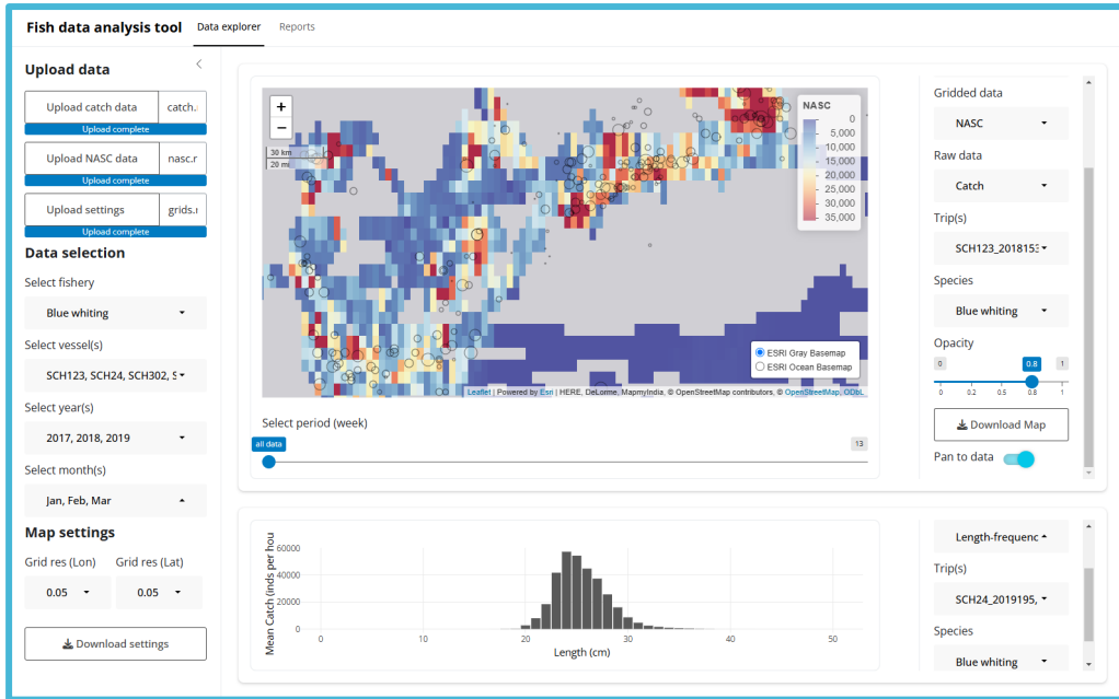
Figure 4.3.1.4. Illustration of dashboard for blue whiting fishery overlaying acoustic backscatter (NASC) with catch and length frequency information.
