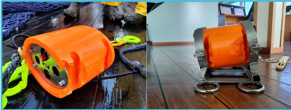
Figure 4.6.6. Broken underwater housing (left) and external casing created (right).
