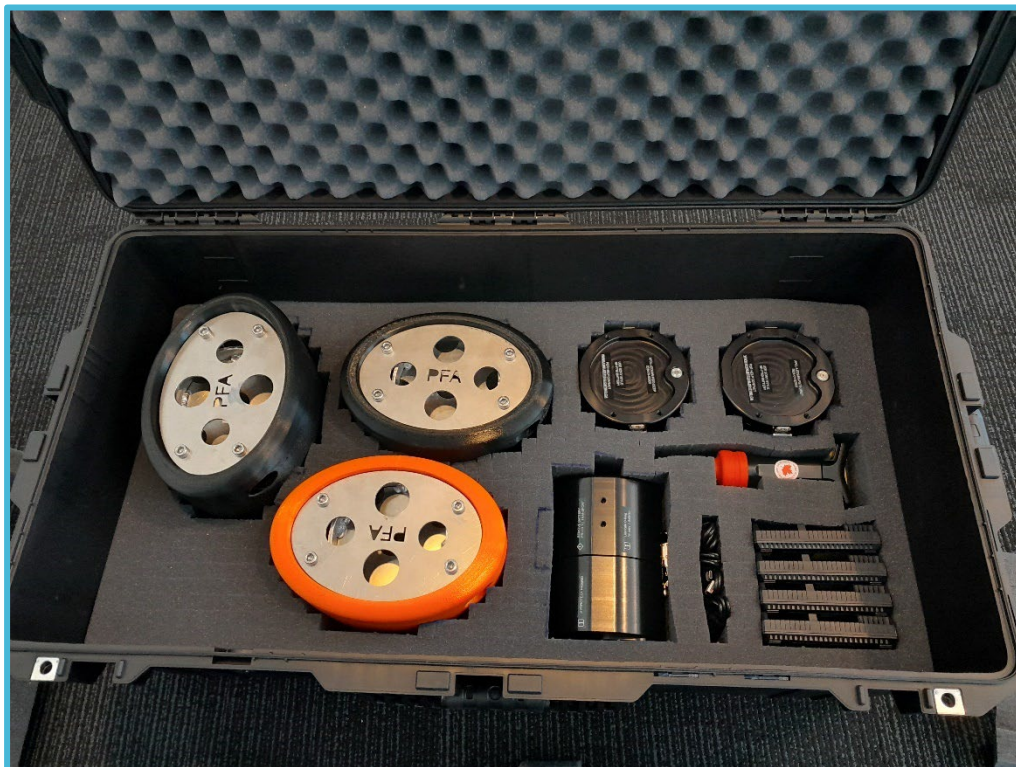
Figure 4.4.1. Deep Sea Trawlviewer kit for two lights and one GoPro unit.
