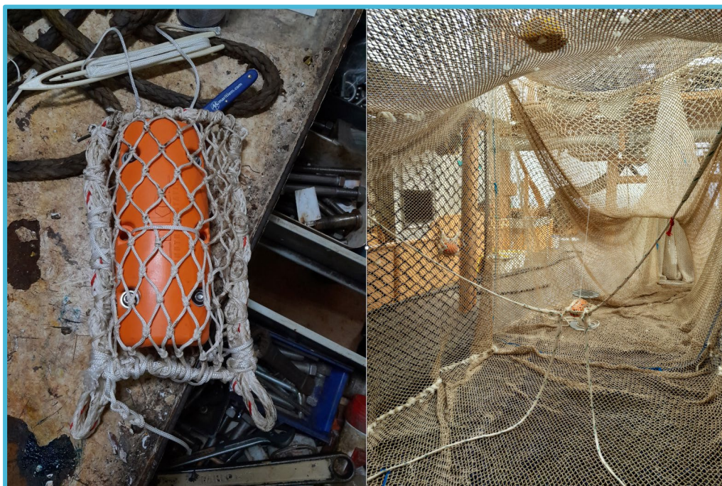
Figure 4.7.3. Oxygen sensor (left), mounted within the codend (right).
